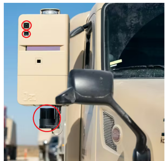
Sensors in cleaning system: WFOV, NFOV Cameras and OT-128 LiDAR
